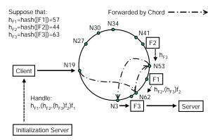
Figure 8. ANON with Chord as the underlying transport network, i.e., ANON over Chord. In contrast, nested encryption is now applied to Chord IDs instead of IP addresses. The IP address of a forwarder is used by a hash function to derive its Chord ID; Chord nodes will forward packets addressed to a forwarder as if it were a request for the object with the same Chord ID.
